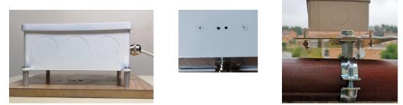
Never cover the two small bottom ventilation holes. Use spacers or similar of at least 10mm. If there is no separation, water will enter the photometer.
